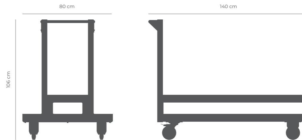
TROLLEY Esc. 1:20 (Weight: 40kg)
