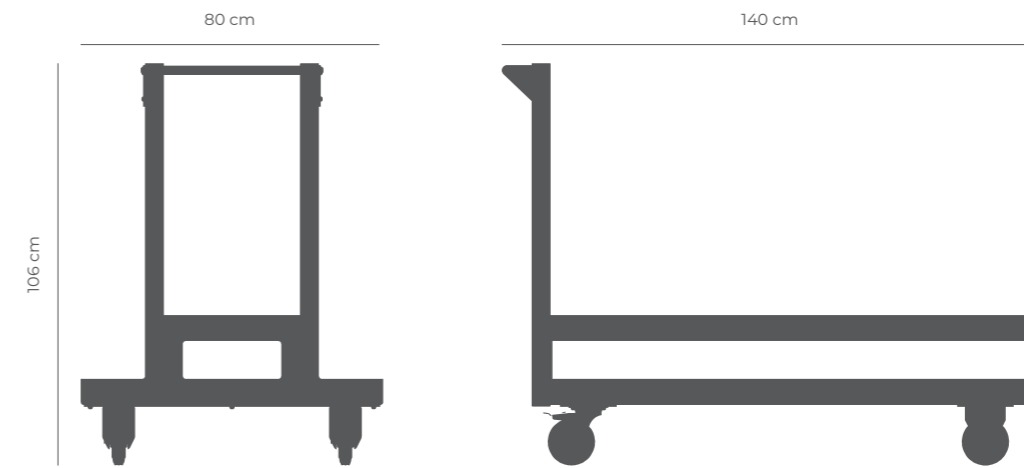
TROLLEY Esc. 1:20 (Weight: 40kg)
