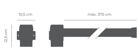
BASIC wall Esc. 1:10 (Weight: 1kg)
